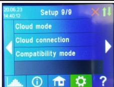
If desired, the settings of the AC ELWA 2 can also be accessed from outside the local network. For this purpose, it is necessary to register the device with serial number and device key in the myPV data cloud: <https://live.my-pv.com/>
