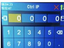
In the case of a control mode with the addition "Manual", the IP address of the signal source must not change during operation [e.g. by a DHCP router], otherwise the AC ELWA 2 will lose the control signal.
